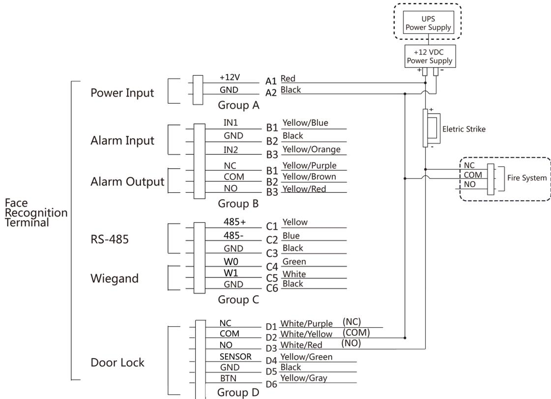
**Figure 4-8 Device Wiring**
