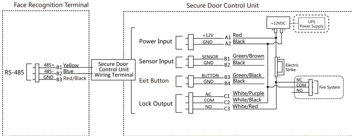
**Figure 4-9 Wiring Diagram**
