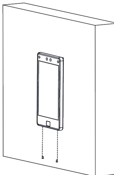
**Figure 3-7 Secure Device**
