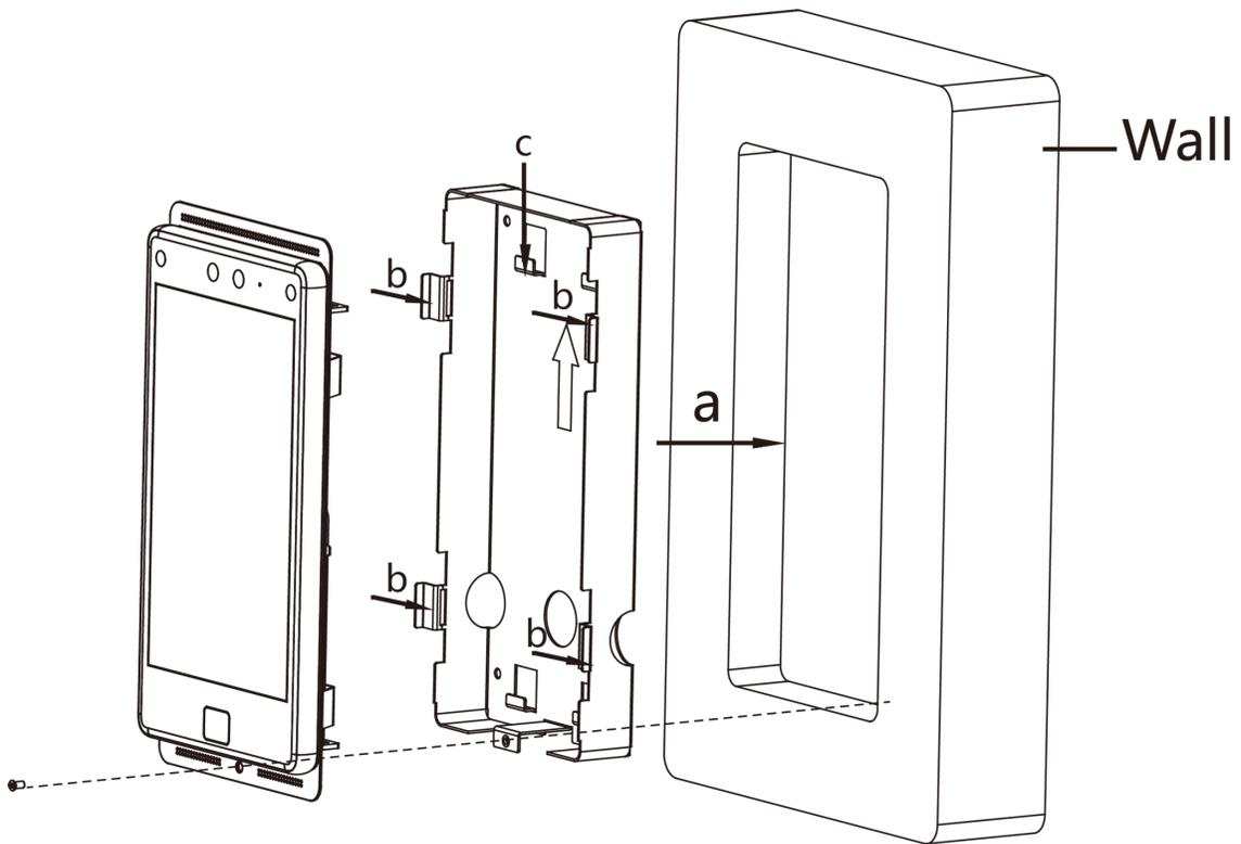
**Figure 3-3 Secure the Combination and the Gang Box**
