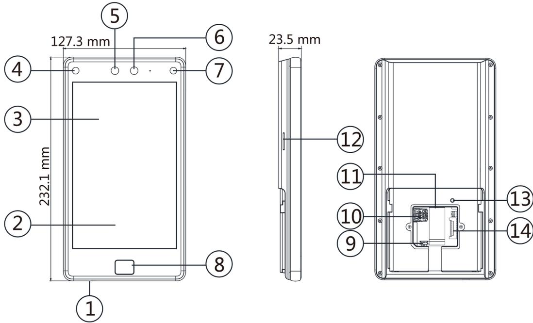
Figure 2-1 Face Recognition Terminal Diagram
