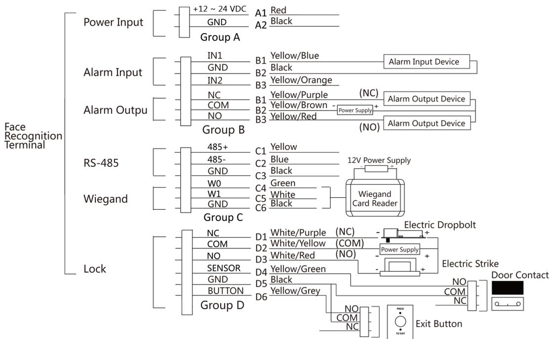
**Figure 4-2 Device Wiring**
