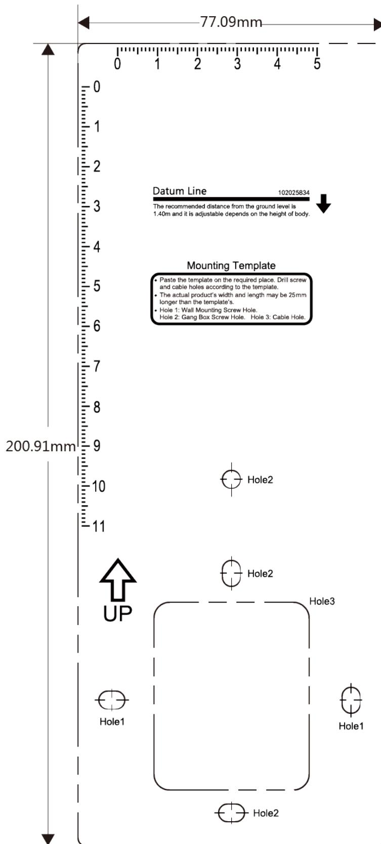
Figure 3-4 Mounting Template
