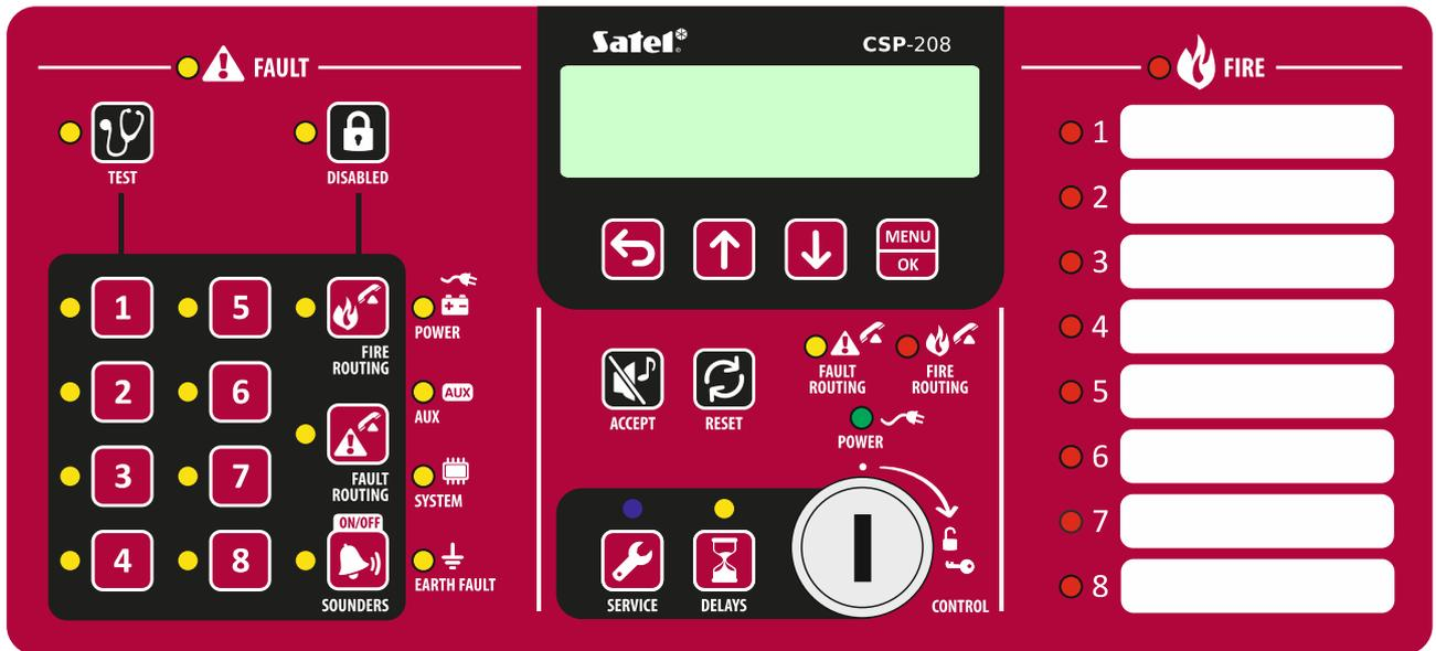
Fig. 2. Front panel of the CSP-208 control panel.
