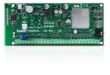
The control panel electronics board is provided with 8 hardwired zones and 4 hardwired outputs. Their number can be increased by connecting the INT–E zone expansion module and INT–O or INT–ORS output expansion module. This allows you to expand the system by adding more detectors, sirens and even actuators (to control the garage door, roller shutters, garden sprinklers).
