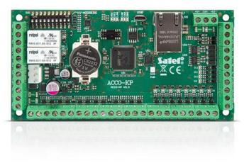
RS-485 bus. In the case of the ACCO NET system, the controller connects to the ACCO–NT access control panel via the RS-485 bus. In turn, communication between the control panel, the system server and the computer with the ACCO Soft configuration program is provided with the use of the TCP/IP protocol.
