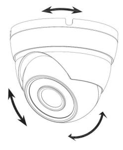
Figure 3-6 Model C adjustment
