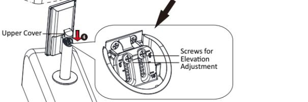
The default elevation angle is 15°. The adjustable elevation angle is from 0 to 15°.
