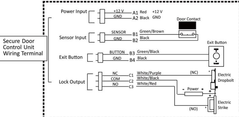
The secure door control unit should connect to an external power supply separately. The suggested external power supply is 12 V, 0.5 A.
